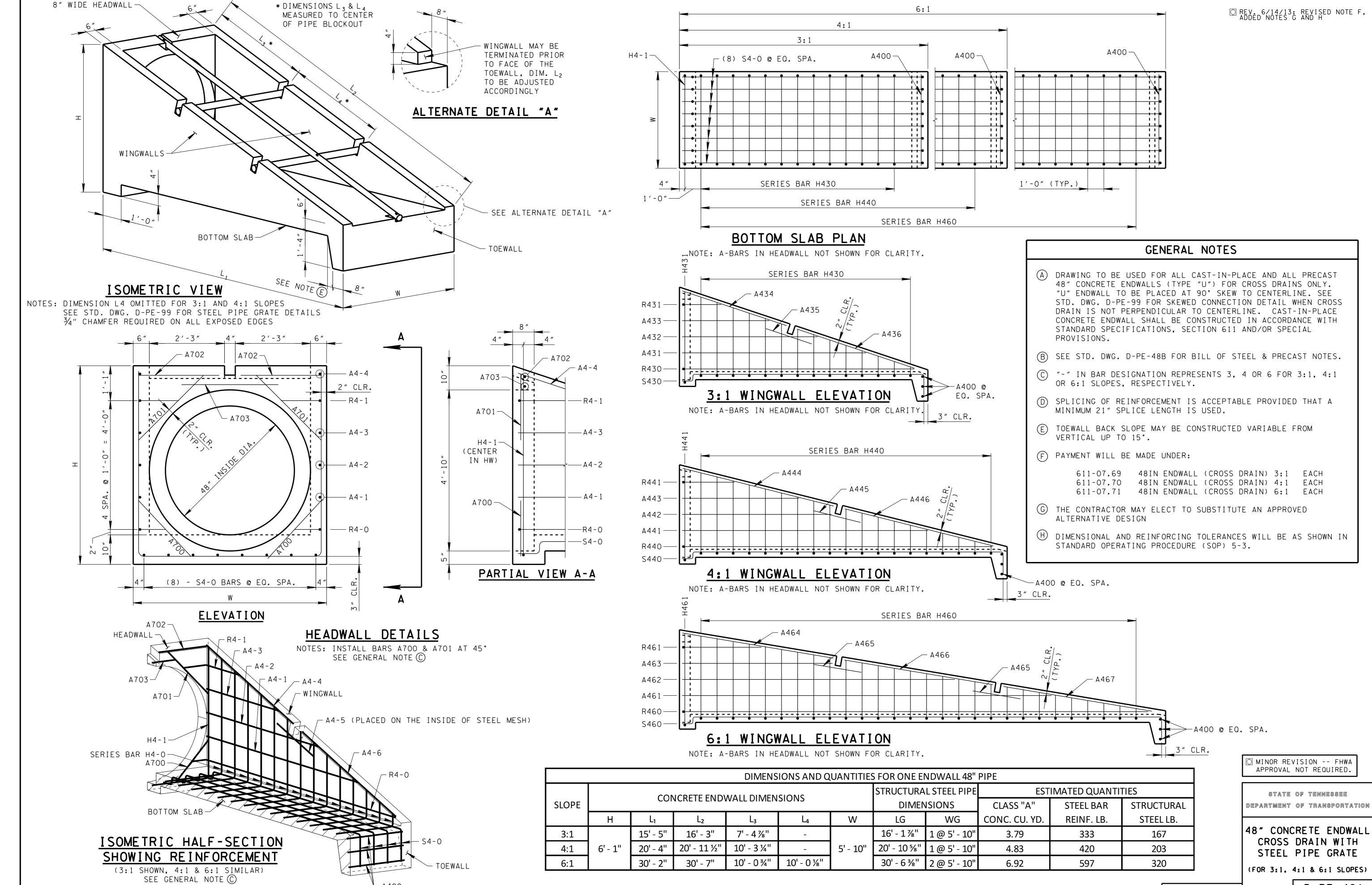
NOTE: SEE STD. DWG. D-PE-99 FOR STRUCTURAL STEEL PIPE DIMENSIONS LG & WG.
